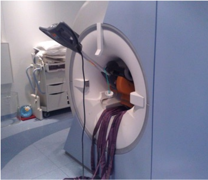
MRI accident on a 1.5T MR system. A floor polishing machine was attracted by the magnetic field. It could only be removed by ramping down the magnetic field. Shown is the back side (head end) of the MRI. Reproduced from: https://commons.wikimedia.org/wiki/File:MRI_accident_on_a_1.5_Tesla_MR_system.jpg
