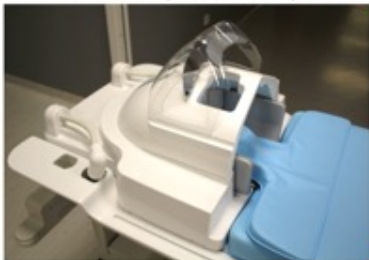
Head coil (32 channels)
